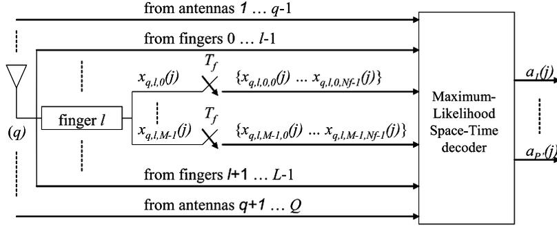
Fig. 1. Schematic representation of the receiver structure during the  $j$ -th symbol duration. The output of the  $l$ -th Rake finger consists of  $M$ -decision variables corresponding to the  $M$  modulation positions for  $l = 0, \dots, L-1$ . The space-time decoder consists of despreading the received frames and performing Maximum Likelihood detection.  $P' = P$  for uncoded systems and IPC (Section III-B) while  $P' = P^2$  for ISC (Section III-A).
