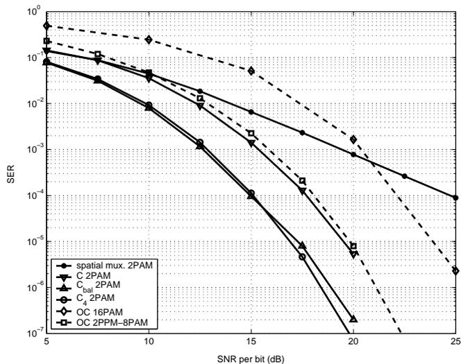
Fig. 5. Performance with 4 transmit antennas, 4 receive antennas and 1 finger Rake.  $C$ ,  $C_{bal}$ , and  $C_4$  are the codes from eq. (17), eq. (26) and eq. (35) respectively while  $OC$  corresponds to the orthogonal code from [2].
