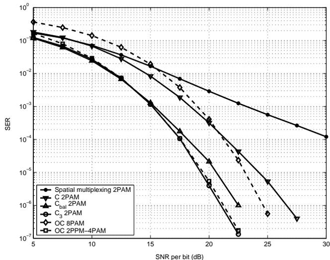
Fig. 4. Performance with 3 transmit antennas, 3 receive antennas and 1 finger Rake.  $C$ ,  $C_{bal}$ , and  $C_3$  are the codes from eq. (17), eq. (26) and eq. (35) respectively while  $OC$  corresponds to the orthogonal code from [2].
