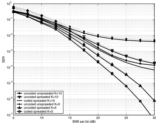
Fig. 9. Performance with  $P = Q = 2$ , 4-PPM-2-PAM and 5 fingers Rake with  $K$  interfering users in an asynchronous environment. The dotted lines associated with each curve correspond to the upper bound based on the Gaussian approximation.
