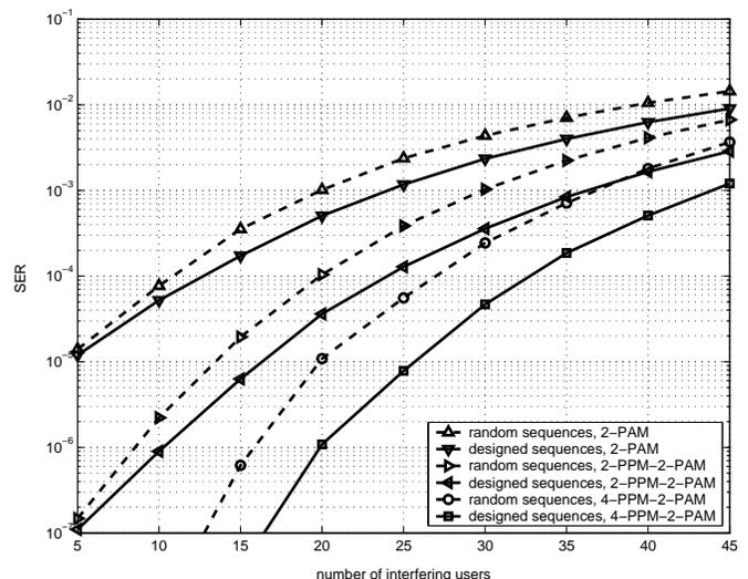
Fig. 10. Performance of IPC from eq. (35) in the presence of MAI with  $P = Q = 2$  and 7 fingers Rake in an asynchronous environment at a SNR of 25 dB. The random and designed sequences correspond to random unitary matrices and to the spreading matrices constructed from eq. (41) respectively.
