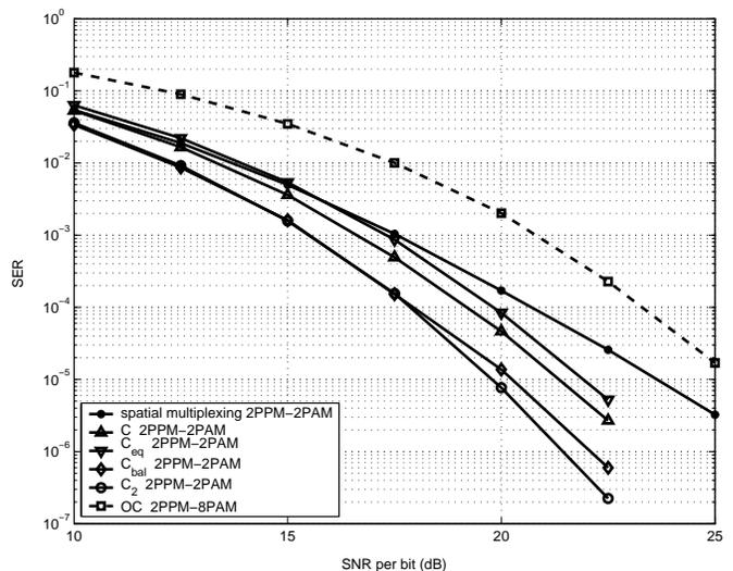
Fig. 3. Performance with  $P=Q=2$  and 5 fingers Rake with 2-dimensional constellations at 4 bits PCU.  $C_{eq}$ ,  $C$ ,  $C_{bal}$  and  $C_2$  are the codes from eq. (21), eq. (22), eq. (27) and eq. (35) respectively while  $OC$  corresponds to the orthogonal code from [1].
