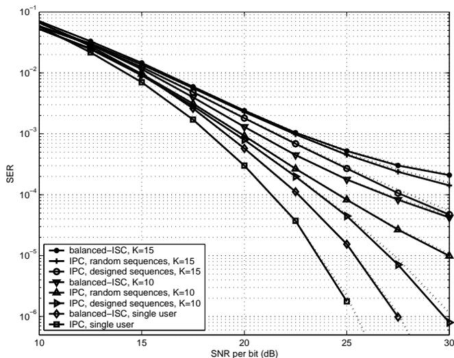
Fig. 8. Performance with  $P = Q = 2$ , 2-PAM and 5 fingers Rake with  $K$  interfering users in a synchronous environment.  $C_{bal}$  and  $C_2$  are the codes from eq. (26) and eq. (35). The dotted lines associated with each curve correspond to the Gaussian approximation.
