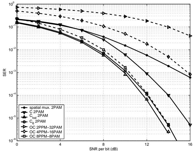
Fig. 7. Performance with 6 transmit antennas, 6 receive antennas and 1 finger Rake.  $C$ ,  $C_{bal}$ , and  $C_6$  are the codes from eq. (17), eq. (26) and eq. (35) respectively while  $OC$  corresponds to the orthogonal code from [2].
