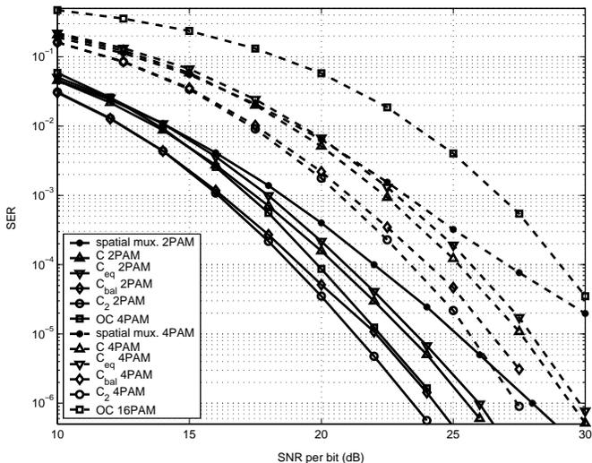
Fig. 2. Performance with 2 transmit antennas, 2 receive antennas and 6 fingers Rake.  $C_{eq}$ ,  $C$ ,  $C_{bal}$  and  $C_2$  are the codes from eq. (21), eq. (22), eq. (27) and eq. (35) respectively.  $OC$  corresponds to the orthogonal code from [1].
