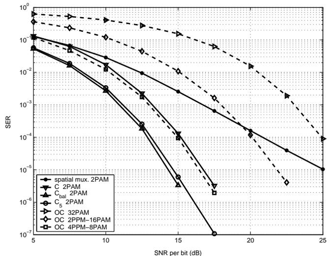
Fig. 6. Performance with 5 transmit antennas, 5 receive antennas and 1 finger Rake.  $C$ ,  $C_{bal}$ , and  $C_5$  are the codes from eq. (17), eq. (26) and eq. (35) respectively while  $OC$  corresponds to the orthogonal code from [2].
