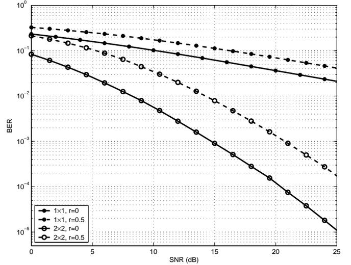
Fig. 4. The impact of IPI on ST-coded MIMO-FSO systems. Nonorthogonal PPM constellations are used and the scalar  $r$  stands for the autocorrelation, of the light waveform, evaluated at the temporal separation between two pulse positions.  $r = 0$  stands for the absence of IPI.
