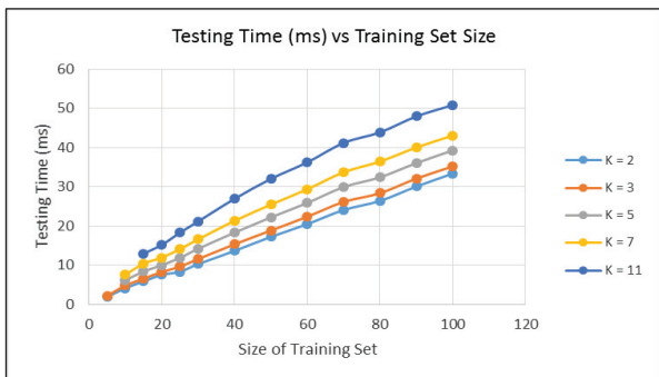
Fig. 5. System Running Time for different training set sizes and k (nearest neighbor) values.
